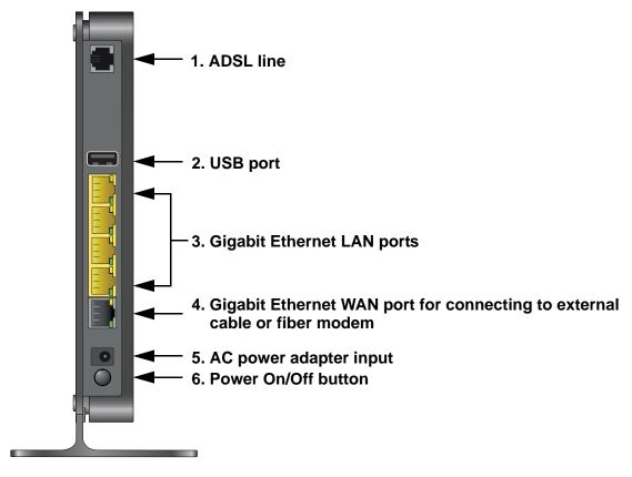
Figure 3. Back panel port connections
